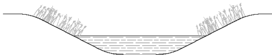
PROPOSED INDICATIVE GRADUAL SLOPING DITCH PROFILE
